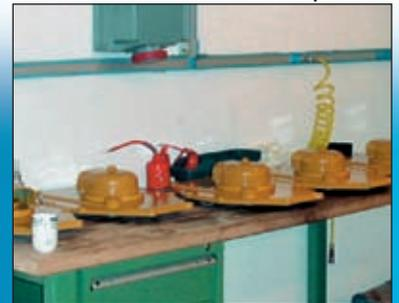
Feeding lines for pneumatic tools along walls or workbenches.
