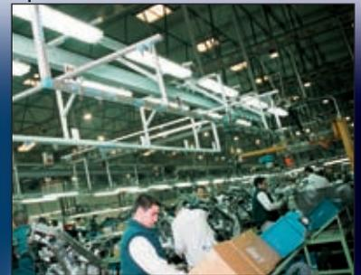
Assembly and production lines built combining aluminium profiles and glider pads.
