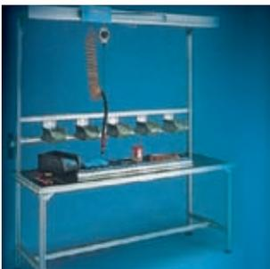
WBA is a workbench equipped for assembly activity operated with pneumatic tools. It is made of anodised aluminium profiles and includes an ATS system for screwdrivers and tools. One of the legs is pressurized acting as both a reservoir and outlet.
