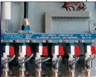
Distribution manifolds integrated on pneumatic control panels for automation.
