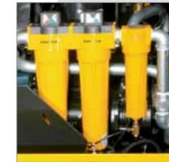
The compressed air is cooled to 7 °C above ambient temperature. Accumulated condensate is able to drain away easily, as the compressed air cooler is installed at an angle, whilst the hot exhaust gasses from the motor are also used to aid condensate evaporation. This design consequently ensures reliable frost prevention during the
